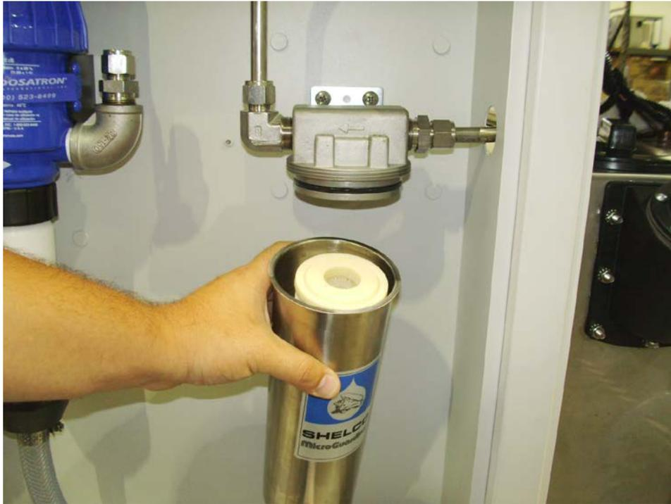
Remove the old O-ring from the filter head and replace with a new one.
